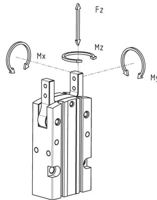
Maximum admissible loads and torques in static conditions
